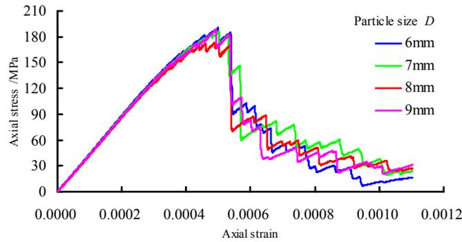
Fig.6 Stress-strain curves of the rock with various particle sizes
