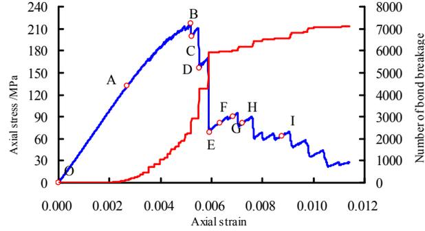
Fig.2 Stress-strain curve during uniaxial compression of rock sample
