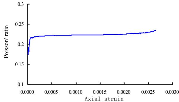
Fig.4 Poisson's ratio of rock sample under uniaxial compression
