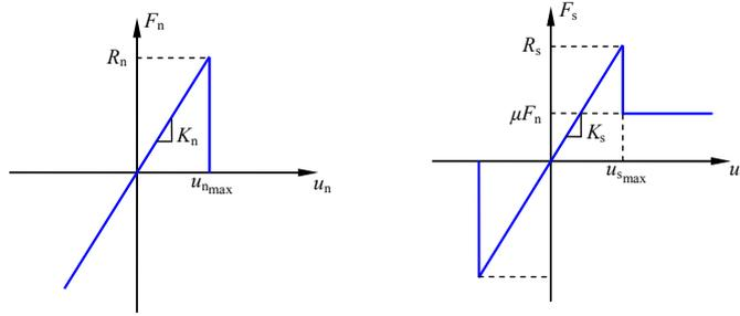
Fig1. Tension and shear constitutive relations of bonded particles and failure criteria
