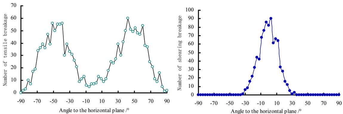
Fig.5 Orientation of tensile and shear failures between bonded particles
