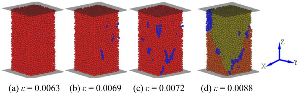
Fig.3 Failure mode of rock sample under uniaxial compression
