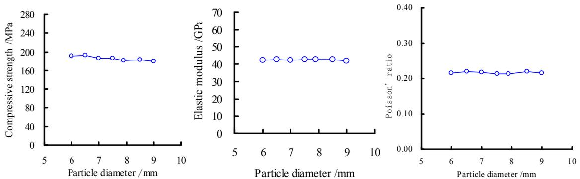
Fig. 7 Elastic modulus, Poisson's ratio and compressive strength with various particle sizes
